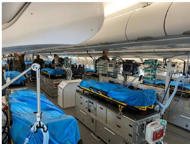
Figure 1. Interior of the Multi Role Tanker Transport Unit 330 with the aeromedical configuration.
