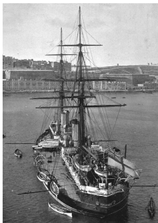
Figure 16. Ironclad battleship HMS Inflexible (11 880 tons, 440 crew, completed 1881), c.1881–1885. 57,58 This ship represents the pace of technical development during this time, which often rendered ships obsolete on entering service – in Inflexible's case, her sails (10 years after Cerberus ), iron armour and muzzle-loading guns in en echelon midships turrets. Inflexible also carried two surgeons and, probably, up to three sick berth 'stewards'. 59
