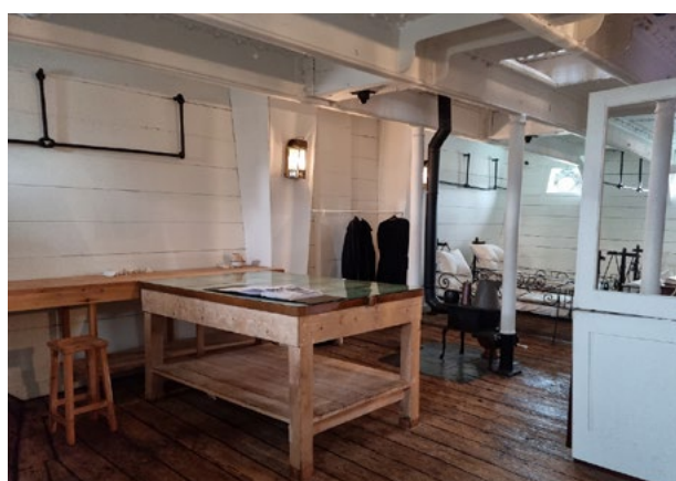
Figure 21. Sickbay HMS Warrior (author, 2022). Note the glass topped operating table (easier to clean than wood before the use of stainless steel), the small stove used for heating and preparing special diets, and the swinging cots for patients. Also note the overhead black iron bars: these were used by the ship's sick berth attendants to sling their hammocks, thereby sharing their living space with their patients at least into the 1940s.
