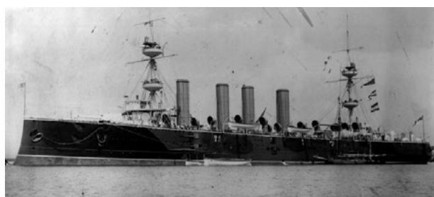
Figure 29. First-class protected cruiser HMS Powerful (14 200 tons, 894 crew, completed 1898), c.1898-1902. 89,90 Note her size (comparable to a pre-dreadnought battleship, see Figure 17) to ensure high speed and long range at the expense of armour and armament. The RN used this type of ship in wartime for battlefleet scouting and its overseas squadrons as flagships and/or wartime commerce protection, typically in remote areas without shore-based medical support. As the Australia Station flagship from 1905 to 1912, Powerful had a sickbay with most likely three medical officers and three sick berth attendants. 91,92
