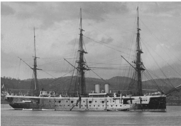
Figure 26. Iron armoured frigate HMS Nelson (7473 tons, 560 crew, completed 1881) undated. 78,79 The RN used this type of ship in its overseas squadrons as flagships, wartime commerce protection and peacetime maritime law enforcement, typically in remote areas for which Nelson still required sails. To these ends, as the Australia Station flagship from 1882 to 1889, she had a sickbay with two medical officers and, probably, up to three sick berth attendants. 80
