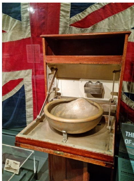
Figures 34 and 35. Officer's cabin washbasin unit, ex-battleship Iron Duke (commissioned 1914) Lyness Museum (author, 2022). RN ships had surprisingly elementary piped freshwater systems even as late as WWI. This led stewards to carry cans of hot water every morning to each officer's cabin to fill the basin seen here. On completing their ablutions, the officer closed the cabinet, thereby emptying the basin into the tank below for removal by the steward. Meanwhile, the crew shared multiple such basins, which may or may not have had piped outlets. Although an improvement for the latter compared to the sailing ship era, these somewhat sketchy hygiene arrangements often endured into WWII.
