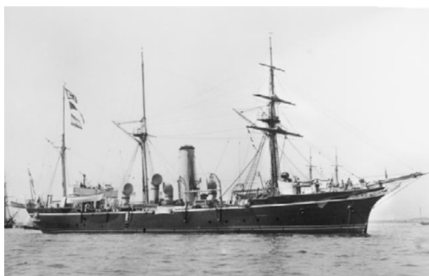
Figure 31. Steel sloop HMS Torch (960 tons, c.106 crew, completed 1894), c.1900. 97,98 Note the sail rig (despite her construction 30 years after Wolverine , see Figure 25), giving her long range in remote areas. The RN used this type of ship in its overseas squadrons for peacetime maritime law enforcement and hydrographic surveying. Torch had a small sickbay with a medical officer and (one would hope) a sick berth attendant.
