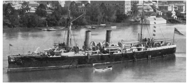
Figure 27. Third-class protected cruiser HMS Wallaroo (2575 tons, 217 crew, completed 1890) at Brisbane, c.1897-99. 81,82 The RN used these smaller cruisers in its overseas squadrons for wartime commerce protection and peacetime maritime law enforcement, for which Wallaroo had a sickbay with a medical officer and a sick berth attendant. 83,84
