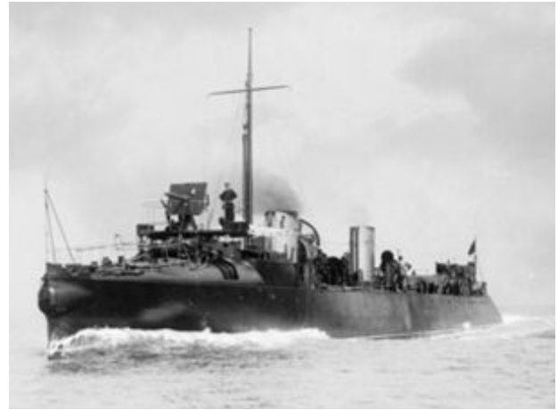
Figure 24. One of the first 'torpedo-boat destroyers', HMS Daring (288 tons, 46 crew, completed 1895), 1897. 72,73 Her small size and high speed (26 kts) reflected their primary role of making night torpedo attacks on enemy battlefleets or defending against them. Combined with their short range and limited seakeeping, these roles precluded their use in Australian waters until the 1910s.
