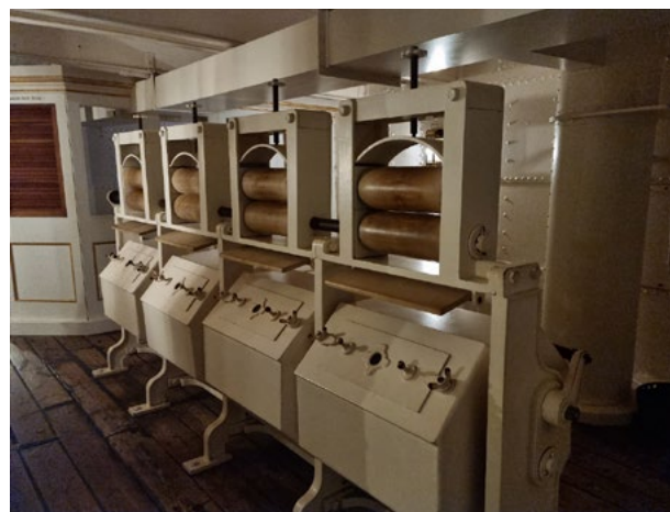
Figure 36. Laundry, HMS Warrior (author, 2022). Dirty clothes and soap were put in the hexagonal boxes and rotated using the hand crank on the right. The clothes were then wrung out using the mangles above, and the process was repeated sans soap to rinse them. They were then hung in a drying room adjacent to the funnel uptakes, ready for the engineers' next watch in the boiler or engine rooms.
