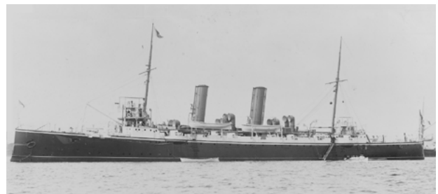
Figure 28. Second-class protected cruiser HMS Cambrian (4360 tons, 318 crew, completed c.1894), c.1894-1902. 85,86 Note her intermediate size compared to third- (Figure 27) and first- (Figure 29) class cruisers, which gave greater capability than the former at considerably less cost than the latter. The RN used this type of ship in wartime for battlefleet scouting and in its overseas squadrons as flagships and/or wartime commerce protection, typically in remote areas without shore-based medical support. As the Australia Station flagship in 1912-13, Cambrian had a sickbay with two medical officers and two sick berth attendants. 87,88
