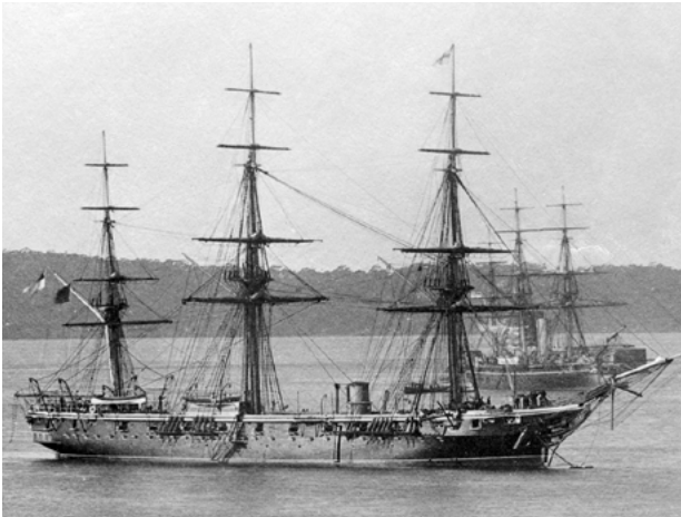
Figure 25. Jason -class wooden screw corvette HMS Wolverene (2424 tons, 240 crew, completed 1864) at Sydney, 1881. 74,75 The RN used this type of ship in its smaller overseas squadrons as flagships, wartime commerce protection and peacetime maritime law enforcement, typically in remote areas without shore-based medical support. As the Australia Station flagship from 1875 to 1882, Wolverene had a sickbay with two medical officers and, probably, two semi-trained sick berth 'stewards'. 76 Her sister Orpheus was wrecked off Auckland while performing the same role in 1863, with the loss of c.166 lives, including the Commander Australia Station, Commodore Sir William Burnett. 77
