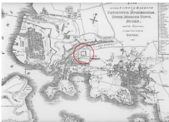
Figure 24. Plan of Plymouth, 1820, showing the naval hospital (circled). 66 Note its location on Mill Lake (since been reclaimed), which permitted direct boat access for the ships. A surrounding high wall reduced the infectious disease risk for the local population and made it harder for convalescents to desert.
