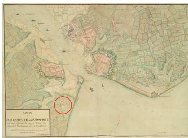
Figure 21. Plan of Portsmouth, 1750, showing Haslar Hospital under construction (circled). 63 Note its location on the Gosport peninsula opposite the dockyard: this permitted direct boat access for the ships, limited the infectious disease risk to the local population, and made it harder for convalescents to desert.
