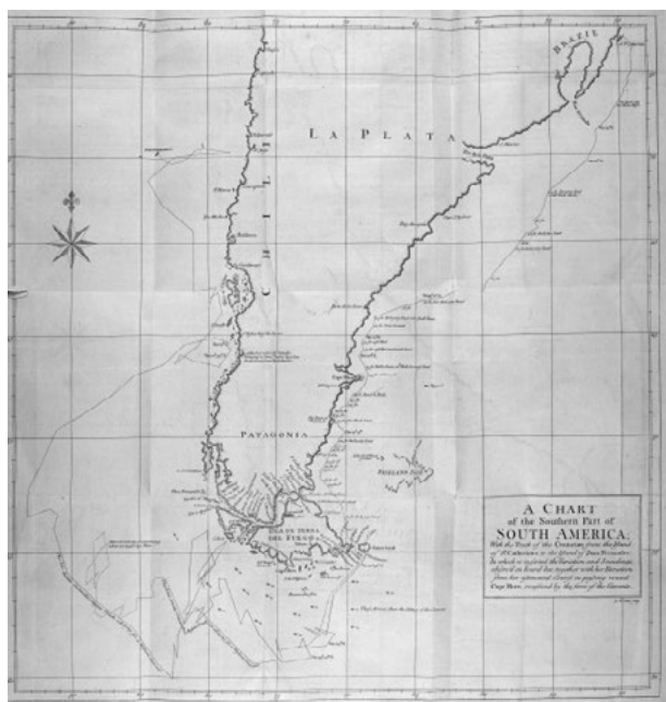
Figure 3. Anson's track chart around Cape Horn, 7 March to 10 April 1741. 34 Note the two tracks resulting from his inability to calculate longitude: one of his estimated route and the other of his actual route, with the former ultimately 300 nautical miles west of the latter. This chart demonstrates how the otherwise avoidable prolongation of sea time exacerbated the scurvy threat to Anson's personnel.
