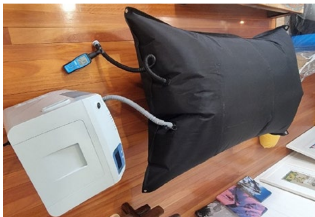
Figure 2 – JAY-10H validation testing configuration with inflated 1000-litre reservoir bag. Schematic configuration is demonstrated in Figure 3.
