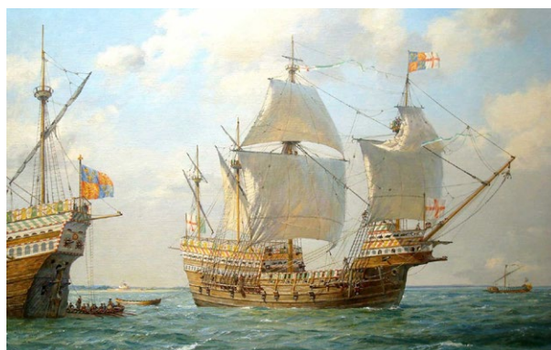
Figure 3. Henry VIII's Mary Rose , c.1520. 20 Note the bluff carrack hull with high (two-storey) fore-and-aft castle, four masts, the anti-boarding nets and (in particular) the hull gunports.
