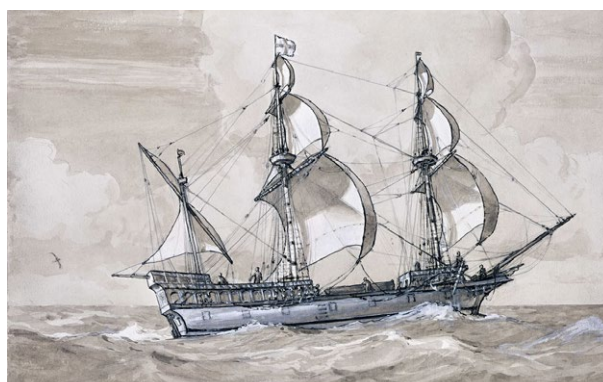
Figure 5. Francis Drake's Golden Hind c.1577. 22 Note the longer and narrower 'race-built' galleon hull, lowered (single-storey) fore-and-aft castles, gunports... and her small size.
