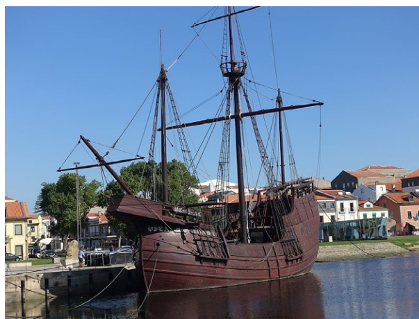
Figure 1. Replica carrack c.1500, Vila do Conde, Portugal. 14 Note the carvel-built hull, three masts each with yards for one or more sails, integral bow and stern castles, and no gunports.
