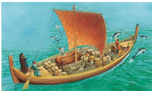
Knorr, c.1200. Note the clinker-built hull, steering oar, open deck without shelter and small crew size. 17
