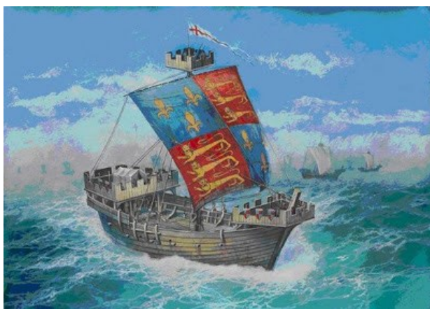
Representation of Edward III's flagship Cog Thomas, which fought the Battle of Winchelsea on 29 August 1350. Note the clinker-built hull with central rudder, weather deck enclosing the hull, and non-integral fore-and-aft fighting castles. Her troops are omitted. 18
