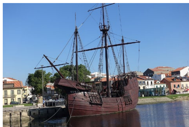
Replica carrack c.1500, Vila do Conde, Portugal. Note the carvel-built hull, three masts with yards for one or more sails, and integral bow and stern castles. 20
