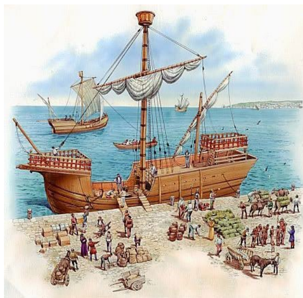
Carrack, c.1400. Note the carvel-built hull with integral fore and after castles, the additional stern fighting castle, two masts with an aft lateen sail, and greater crew size. 19
