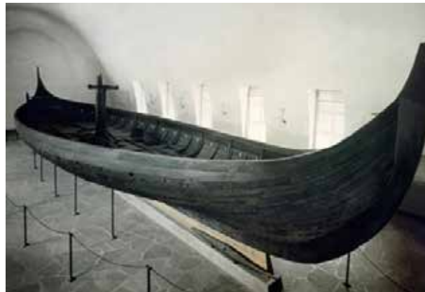
Gokstad ship found 1880, dated c890 CE. 41 Note the oar ports, loose deck planking and absence of decorative carving. The bow is to the right.
