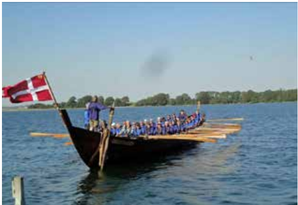
Nydam ship replica Nydam Tveir; 34 Note the steering oar on the starboard quarter and absence of a sail.
