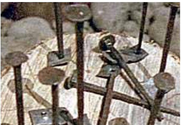
Replica Viking Age iron boat rivets and washers. 35 Each rivet was inserted from the outside of the hull while red-hot so the bottom edge of the uppermost plank or 'strake' overlapped the top edge of the strake below. A washer was placed over each rivet inside the hull and hammered in place.
