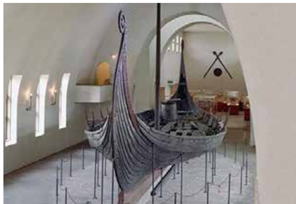
Oseberg ship found 1903, dated c820 CE. 39 Note the bow decorations, loose deck planking and absence of rowing thwarts.
