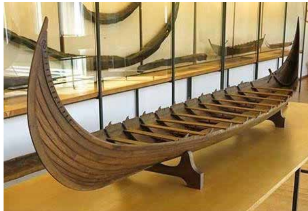
Model, Kvalsund ship, found 1920, dated c690 CE. 38 Note the rowlocks and thwart, and absence of a mast and sail. The bow is to the left.
