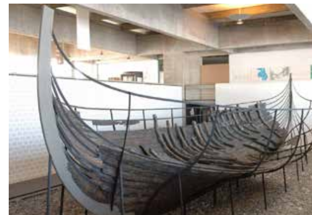
'Skuldelev 1' knarr, one of five vessels found near Roskilde, Denmark in 1962, dated 1030 CE. 44 Note the broader beam and heavier lines compared to the Gokstad ship.
