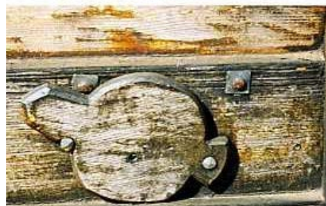
Gokstad ship oar port covers. 42 The port slot at 10 o'clock in the upper photo is for the oar blade.
