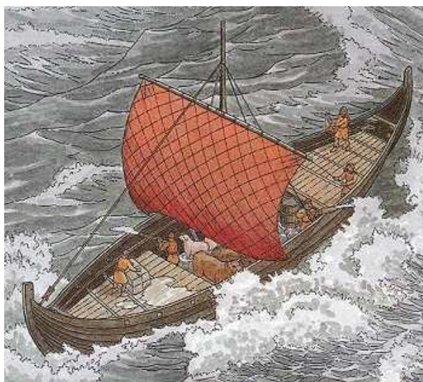
Representation of a knarr in bad weather. 46 Note the absence of crew shelter, the knee-deep water in the cargo area amidships—and the two bailers.
