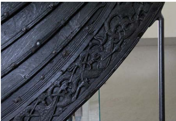
Oseberg ship closeup. 40 Note the stem carvings and rivets.
