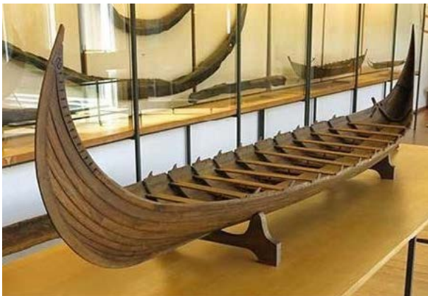
Model, Kvalsund ship, found 1920, dated c690 CE. 38 Note the rowlocks and thwarts, and absence of a mast and sail. The bow is to the left.
