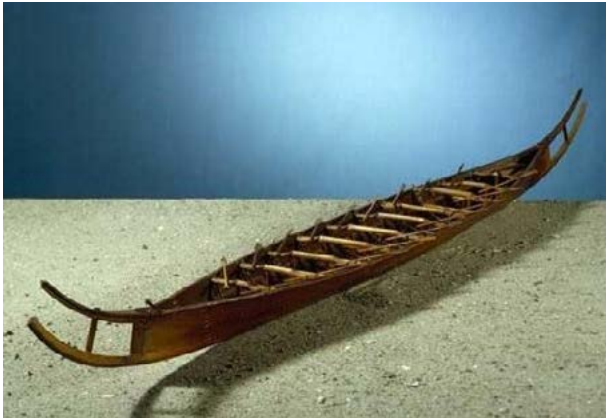
Hjortspring boat model, National Museum of Denmark. 32 Note the combination rib/paddle thwarts. The purpose of the projections at either end remains unknown.
