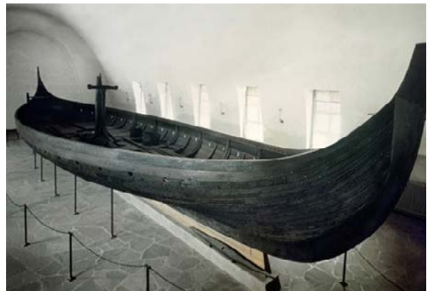
Gokstad ship found 1880, dated c890 CE. 41 Note the oar ports, loose deck planking and absence of decorative carving. The bow is to the right.
