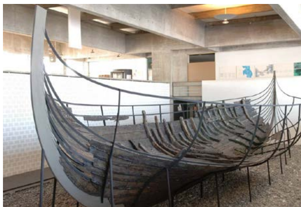
'Skuldelev 1' knarr, one of five vessels found near Roskilde, Denmark in 1962, dated 1030 CE. 44 Note the broader beam and heavier lines compared to the Gokstad ship.
