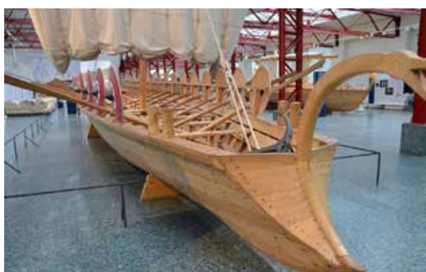
Forward view, replica Roman navis lusoria, c. 300 CE, Mainz Museum Germany. 30 Used on the Rhine as a troop transport. Note the faux ram bow.
