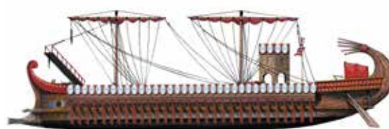
Roman quadreme ( bireme with two rowers per oar), c. 260 BCE. 26 Note the heavier overall build compared to the trireme, the corvus forward and the archery tower aft. Quinqueremes were similar but with five rowers for three banks of oars.
