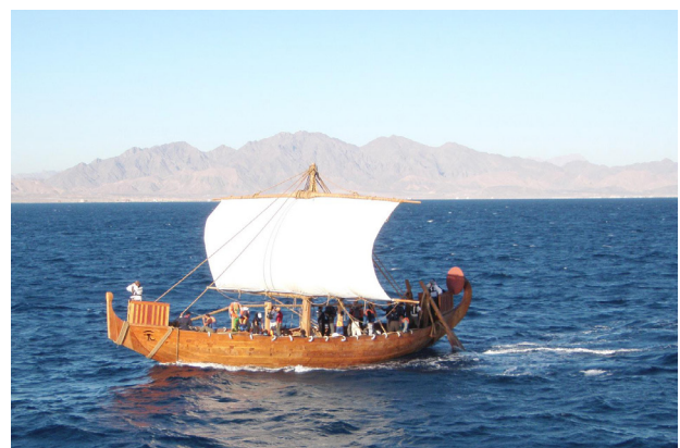
Replica Egyptian seagoing 'Byblos' ship Min of the Desert, from c1500 BCE. 33 Note the sail, the fore-and-aft anti-hogging truss, and places for oars.
