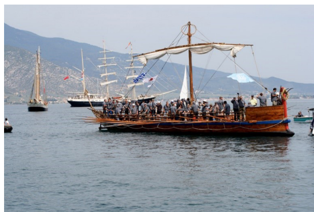
Replica Greek Pentecontor Argo from c800 BCE. 43 Note the rather petite ram bow and single bank of oars.
