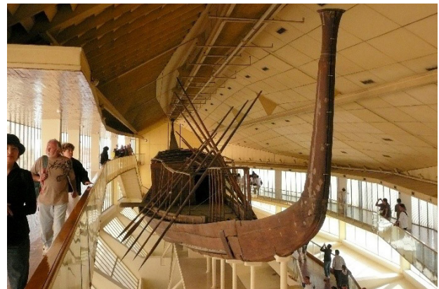
Khufu ship, dated c2500 BCE, bow view 30 . She is 43.6m long, 5.9m beam, displaces 45 tons, and is one of the oldest, largest, and best-preserved vessels from antiquity. She was found in a pit at the Giza pyramid complex, disassembled into 1223 pieces but otherwise complete, in 1954. 31
