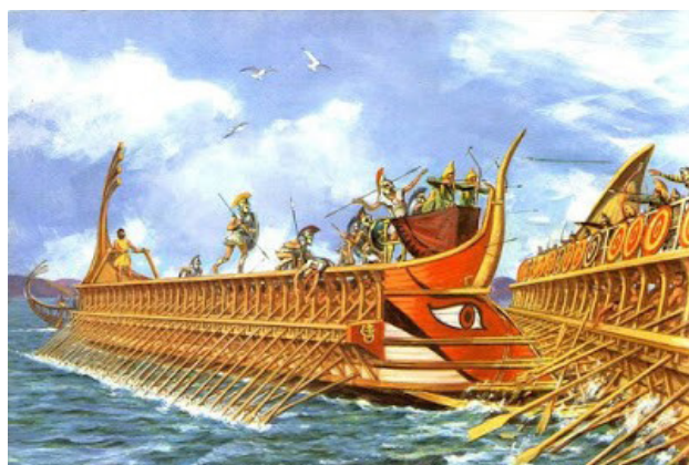
Greek trireme in action, 480 BCE. 46 Note the absence of the mast and sail, and the hoplites and archers on the upper deck. Also note the oblique ramming angle, which not only holes their opponents' hull, but also breaks more oars (thereby also injuring more rowers) compared to perpendicular 'T-boning'.
