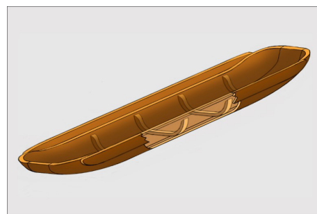
Diagrammatic representation of a northern European dugout, c1300 BCE. 61 The cutaway shows how the parent log has been split in half, with a plank inserted between to increase beam and transverse ribs to hold them together. Also note the lack of a keel. (Author)
