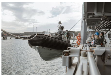
Launching a RHIB, Unit Readiness Evaluation, HMAS Toowoomba, 2019. 48 The difficulties, dangers and limitations associated with moving stretcher cases via this means should be apparent.
