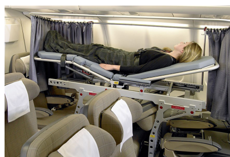
Stretcher fit, commercial passenger aircraft. 37 Note how one stretcher case uses the same space as six seats.
