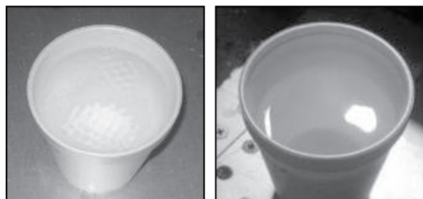
Figure 8. A series of photos of a fluid filled container sitting on the floor of an airborne C-130 J AME aircraft. The photo to the left shows the pronounced vibration in the propeller line of the aircraft. The photo on the right demonstrates minimal disturbance in the aft end of the fuselage, adjacent to the DCI patient. Consideration should be given to place the DCI patient stretcher in the position with the least vibration.
