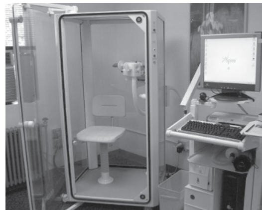
Figure 8: A whole-body plethysmograph. For infants it is necessary that a parent or carer sits in the box nursing the infant. the healthy parent will tolerate SO_2 of 15% with no difficulty. Photo Joe Mabel-the swedish Hospital Ballard Campus, seattle, Washington. http://en.wikipedia.org/wiki/File:Body_Plethysmography_chamber_01.jpg
