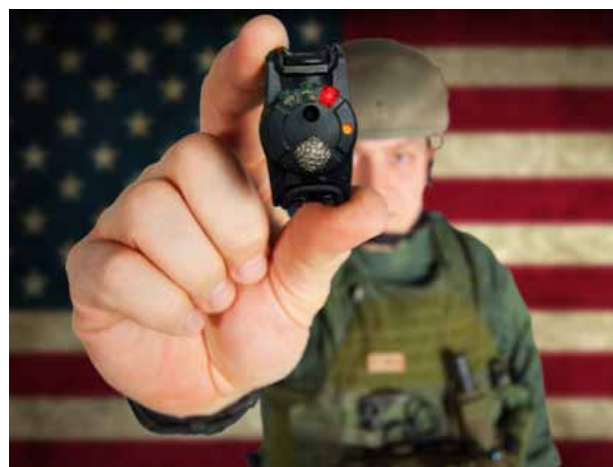
Image 3: Blackbox Biometrics B3 Blast Gauge showing activation of Red Indicator Light. (Photograph courtesy of BlackBox Biometrics Inc.)
