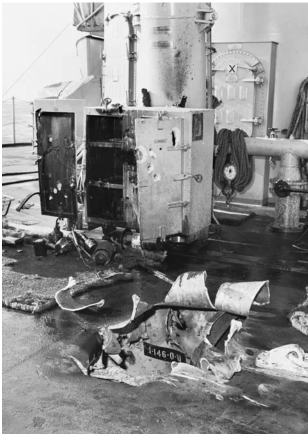
Shell hit, HMAS Perth , 18 Oct 67. Entry hole in 01 deck forward of Mount 52 after ricochet. (AWM NAVY14773)
