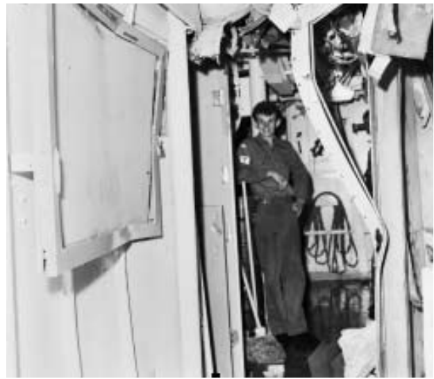
Unidentified (and very young) stoker, and below-deck damage from shell hit, HMAS Perth , 18 Oct 67. The shell exploded in the registered publications vault on the right (note the blown-out door frame). Also note the width of the passageway. (AWM NAVY14761)
